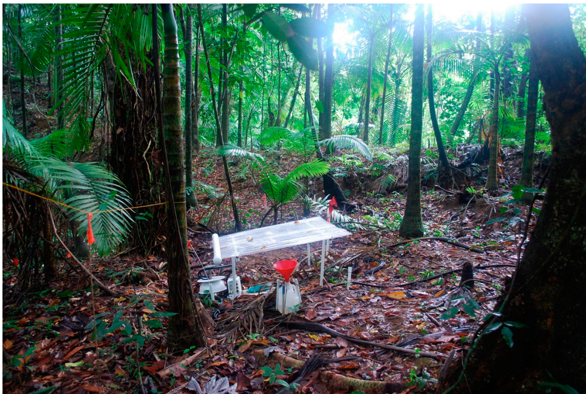
Figure 5. Throughfall exclusion shelter installed in the Luquillo Experimental Forest. Photograph by Tana E. Wood.
