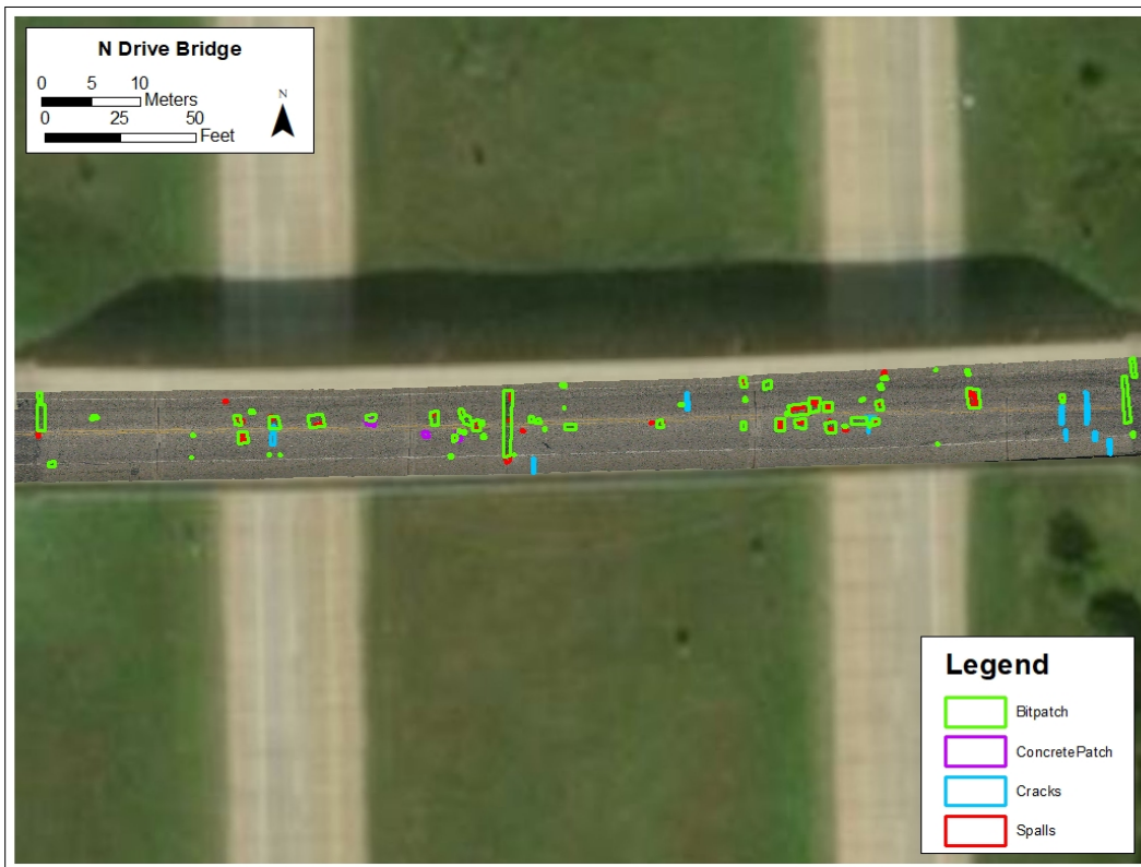
Figure 9. Identified distresses on the N Drive Road bridge.
