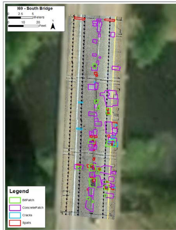
Figure 12. Identified distresses on the I-69 South bridge.
