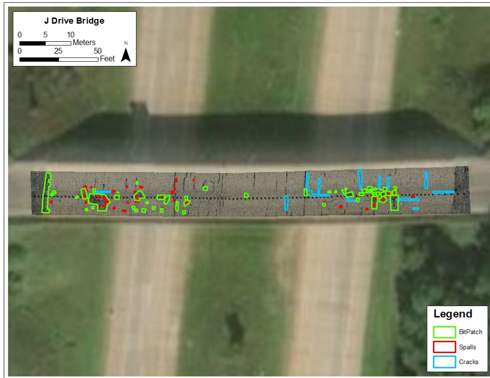
Figure 8. Identified distresses on the J Drive Road bridge.
