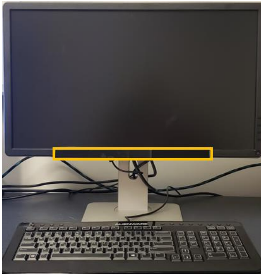
Figure 4 Monitor set up with mounted Tobii X3-120 Eye Tracker (outlined in gold).
