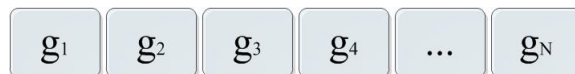
Figure 2.1: In standard GA, a chromosome (code) is a string of genes that represent a solution
