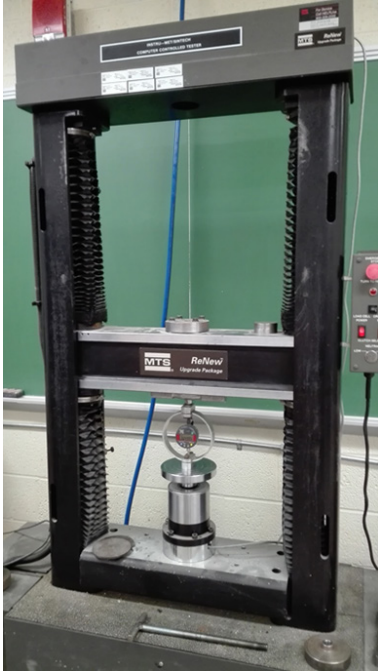
Figure 34: Press used for the calibration of the CPT device, laboratory of geotechnics of the Geological & Mining Engineering & Science department of the Michigan Technological University
