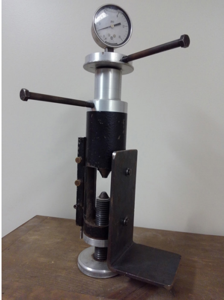
Figure 21: Point Load Test device from Michigan Technological University, department of Geological & Mining Engineering & Science
