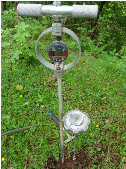
Figure 33: Cone Penetration Test (CPT) device on the left and Shear Vane device on the right. Machines from the Geological & Mining Engineering & Science department of the Michigan Technological University
