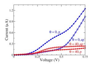
FIG. 5. (Color online) Comparison of *I-V* characteristics for parallel (*P*) and antiparallel (*AP*) magnetic alignments of the Ni contacts, for  $\theta$ =0° and  $\theta$ =40°.
