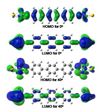
FIG. 4. (Color online) HOMO-LUMO plots for the two extreme cases  $\theta$ =0 and 40° of parallel spin configuration. Blue(black) and green(gray) are used to indicate the positive and negative sign of the wave function. From these HOMO-LUMO plots, it is evident that the current is mainly controlled by the overlap of molecular orbitals on backbone of the molecule.
