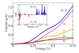
FIG. 3. (Color online) Current-voltage characteristic of the molecular device shown in Fig. 1, for different rotation angles  $\theta$  of the central benzene molecule, for the case of parallel magnetic alignment of the Ni contacts. Inset: Total density of states (DOS), for the two extreme cases  $\theta$ =0 and 40°, near the Fermi level (zero of energy).
