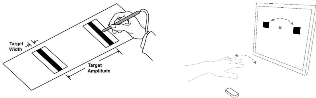
Figure 1.4 traditional Fitts's task, image from (MacKenzie, 1992) (left), proposed setup for air gesture equivalent task (right)
