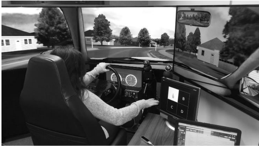
Figure 3.3 driving simulator setup, visual display monitor with webcam, and LEAP Motion.
