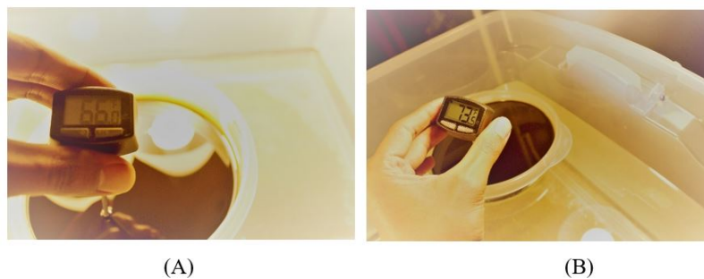
Figure 3.3. Oil Temperature Measurements (A) Before Heating (B) After 3 Hours Heating
