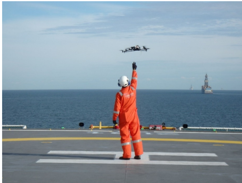
Figure 1.2. UAS Deployment for offshore platforms routine inspections
