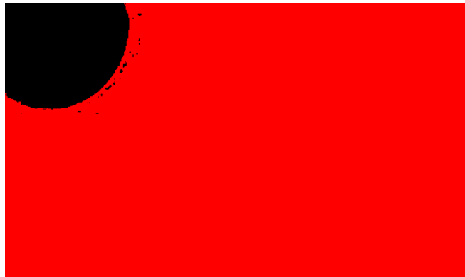
Figure 4.11. RGB image classification where red is water and black is oil
