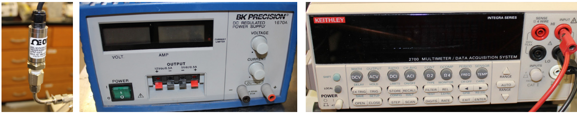
Figure 4.3: Pressure transducer - PX309-015AV model (left) with the DC power source (mid) and the Keithley 2700 multimeter (right).
