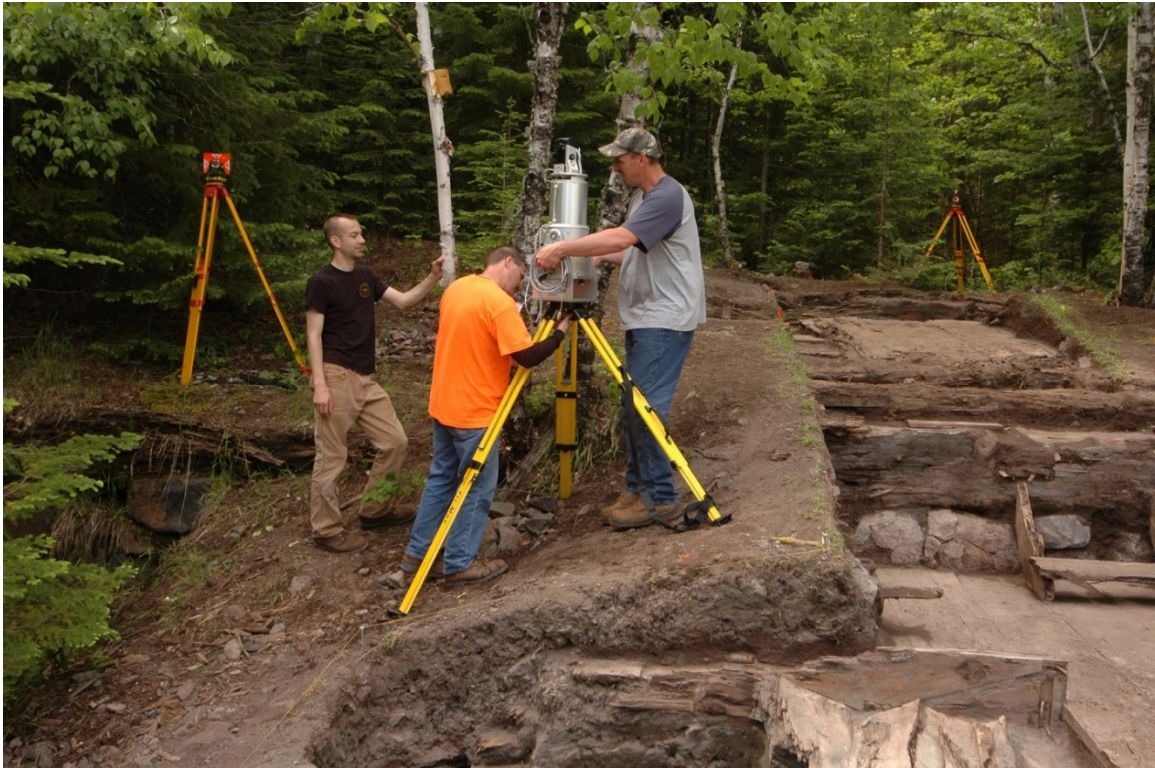
Figure 3.3. Setup of Riegle long-range terrestrial laser scanner. (Image by author, 2011)
