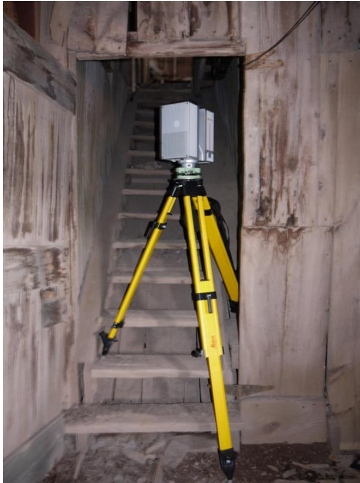
Figure 3.6. Leica HDS7000 Laser Scanner in second floor doorway Champion #4 Shaft House. (Image by author 2013)
