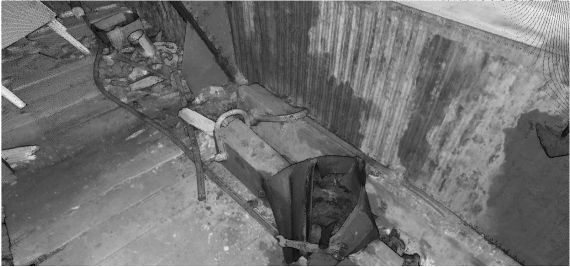
Figure 3.7. Point cloud image from HDS7000 laser scanner. Scanning was performed in a dark environment with no additional lighting. (Image exported from Leica Cyclone 7 software).
