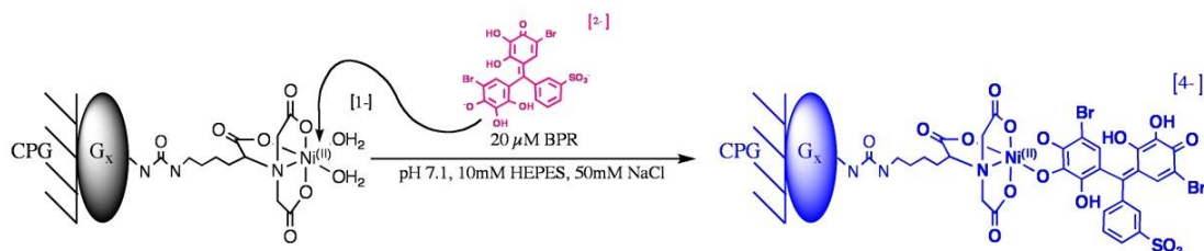
Figure 2.8. A molecule of BPR chelating a nickel metal center of a modified CPG molecule.
