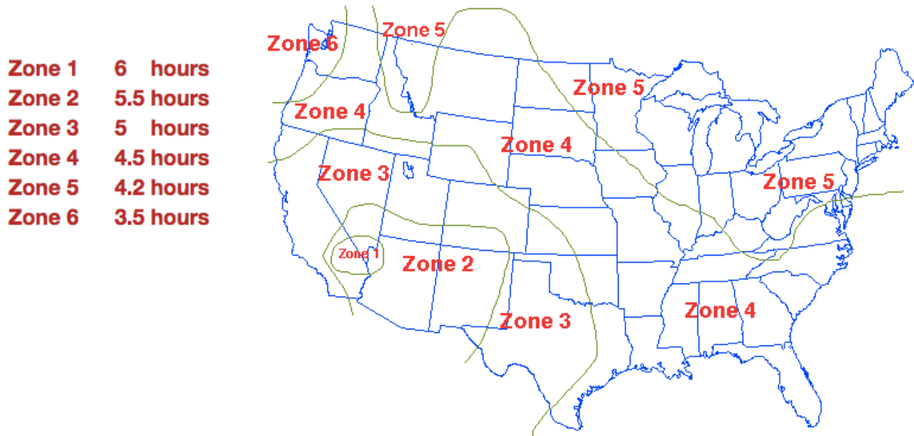
Figure 6 Solar Insolation Map of sun hours/day in the United States (from "Solar Insolation Map", 2017).
