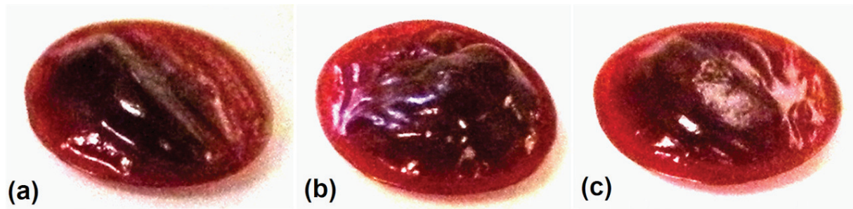
Figure 8. Samples treated with a total of 16 s exposure time (4 s exposures, with a 2 s pause between two consecutive exposures) at three exposure distances, namely (a) 25 mm, (b) 30 mm and (c) 40 mm.
