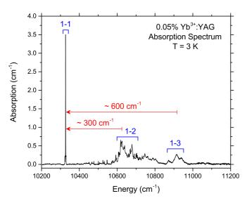
FIG. 1. Absorption spectrum of 0.05% Yb<sup>3+</sup>:YAG (unpolarized) for the  ${}^2F_{7/2}$  to  ${}^2F_{5/2}$  transition at T = 3 K. Indicated are the transitions from the lowest level of  ${}^2F_{7/2}$  (1) to the three Stark levels of  ${}^2F_{5/2}$ .
