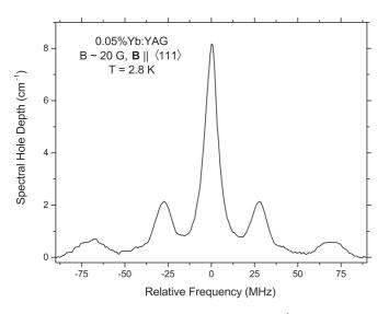
FIG. 8. Example of a spectral hole in 0.05% Yb<sup>3+</sup>:YAG at 2.8 K with a field of  $\sim$ 20 Gauss along  $\langle 111 \rangle$ , showing strong electronic spin-flip sidebands.
