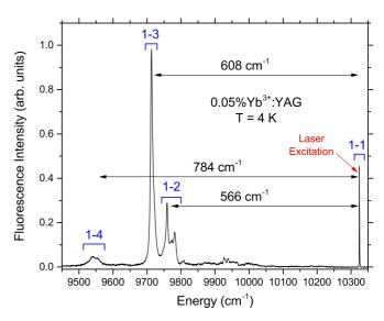
FIG. 2. Fluorescence spectrum of  ${}^2F_{5/2} \rightarrow {}^2F_{7/2}$  for 0.05% Yb<sup>3+</sup>:YAG at T = 4 K. To avoid spectral hole burning, the spectrum was measured by exciting the  ${}^2F_{5/2}$  (1) level at 10 324.5 cm<sup>-1</sup> with a laser. Energy differences were measured between the peaks of the emission intensity for each transition.
