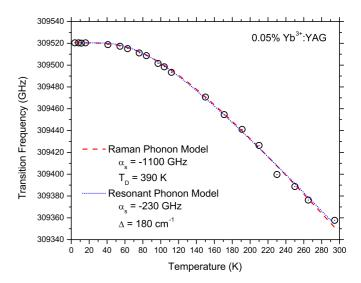
FIG. 5. Thermal line shift of the  ${}^2F_{7/2} \rightarrow {}^2F_{5/2}$  transition frequency in 0.05% Yb<sup>3+</sup>:YAG. The data were fit using the models described by Eqs. (2) and (3) with values for the resulting fit parameters shown.
