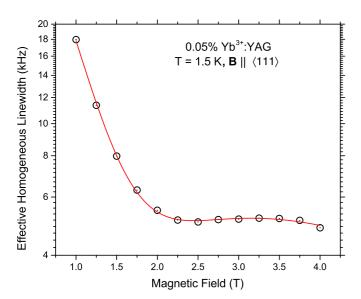
FIG. 11. Effective homogeneous linewidth dependence on magnetic field strength in 0.05% Yb<sup>3+</sup>:YAG at 1.5 K with B $||\langle 111\rangle$ . Symbols correspond to experimental data. The solid line is a fit to the spectral diffusion model described by Eqs. (8)–(10).
