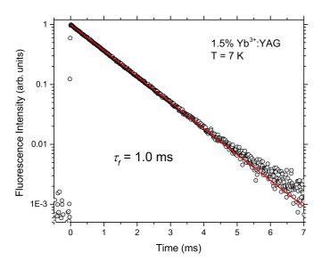
FIG. 7. Fluorescence lifetime decay of the  ${}^2F_{7/2}(1) \rightarrow {}^2F_{5/2}(1)$  transition for 1.5% Yb<sup>3+</sup>:YAG at T=7 K. The solid line is a single-exponential fit to the data with a lifetime of  $T_1=1.0$  ms showing good agreement.
