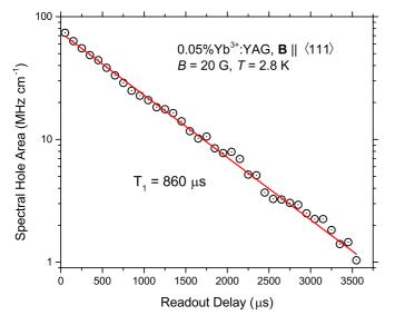
FIG. 9. Measured spectral hole decay in 0.05% Yb<sup>3+</sup>:YAG at  $T=2.8 \,\mathrm{K}$  with a field of B=20 Gauss along the  $\langle 111 \rangle$  axis. The solid line is a single-exponential decay fit to the data showing good agreement and providing a  $^2F_{5/2}(1)$  excited state lifetime of  $T_1=860 \,\mu\mathrm{s}$ .
