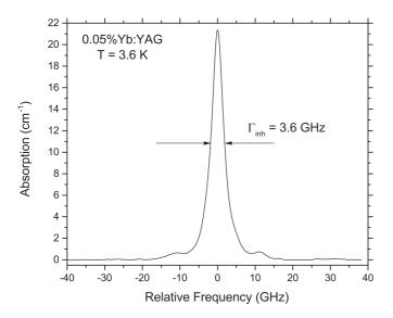
FIG. 3. Laser-absorption spectrum of the  ${}^2F_{7/2} \rightarrow {}^2F_{5/2}$  transition at 968.571 nm (vacuum) in 0.05% Yb<sup>3+</sup>:YAG at T=3.6 K revealing an inhomogeneous linewidth of 3.6 GHz. Also noticeable in the spectrum are small satellite lines due to perturbed Yb<sup>3+</sup> sites in the crystal.
