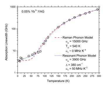
FIG. 6. Thermal broadening of the inhomogeneous line of the  ${}^2F_{7/2} \rightarrow {}^2F_{5/2}$  transition in 0.05% Yb<sup>3+</sup>:YAG. The data were fit using the models described by Eqs. (4) and (5) with values for the resulting fit parameters shown.
