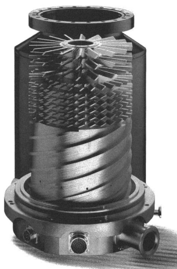
Figure 2-10. A compound turbomolecular pump with the rotor shown. 25
