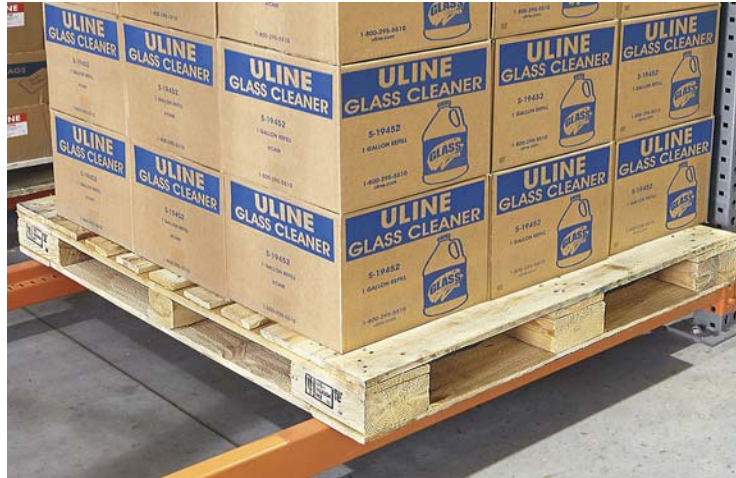
Figure 2.2: Most commonly used block pallet in the industry [8] [26].
