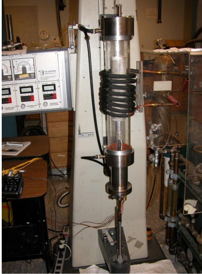
Figure 8: Bridgman furnace assembly used for directional solidification experiments
