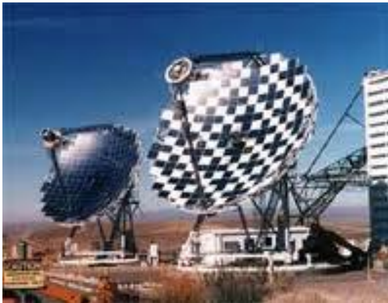
Figure 27. Test Bed Concentrators at Sandia, showing a fully cantilevered drive system.
