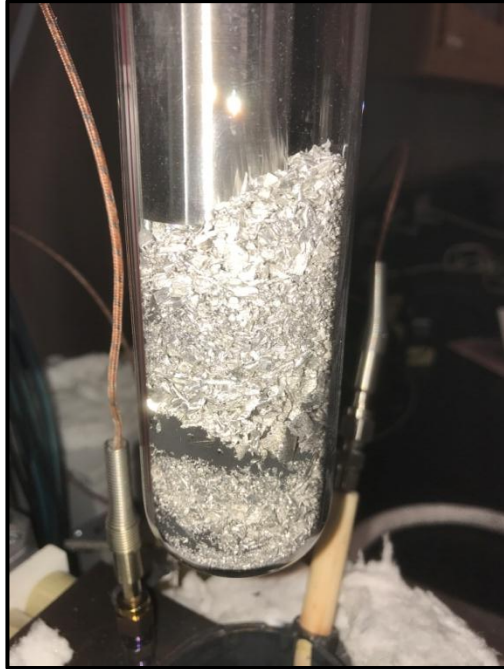
Figure 19: Improper layered MWCNTs in Test tube
