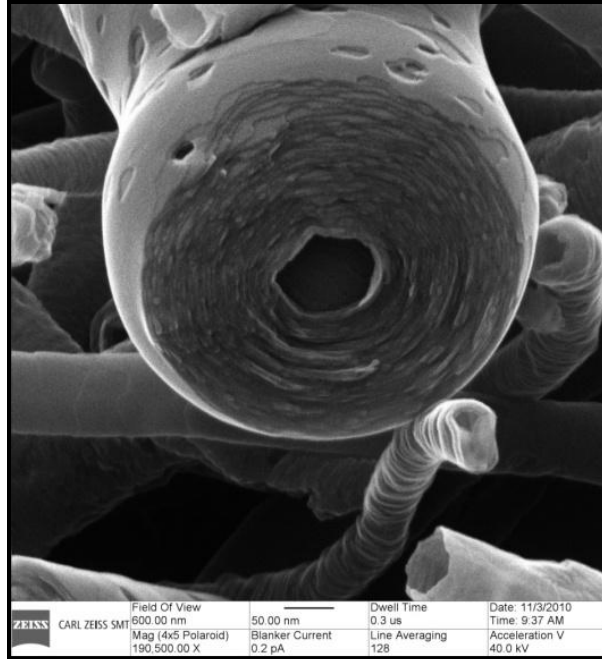
Figure 6: SEM image of MWCNT
