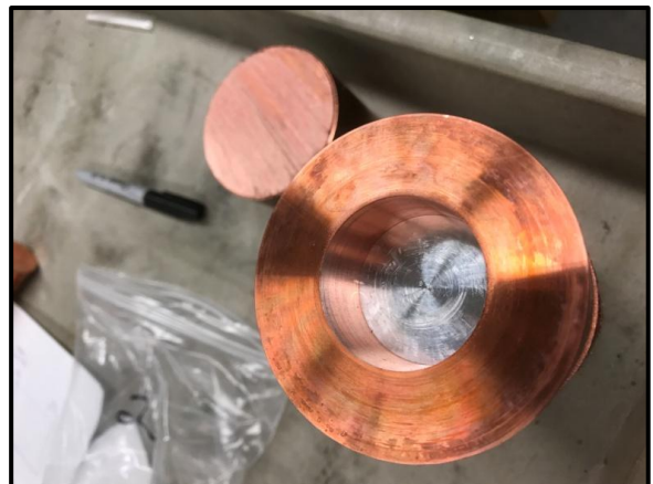
Figure 27: Mg/MWCNT composite embedded in Copper Billet
