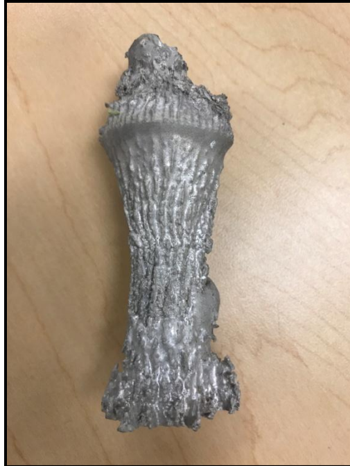
Figure 17: Magnesium billet processed using Electromagnetic Induction
