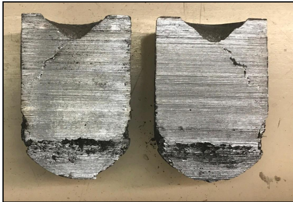
Figure 21: Defective Mg/MWCNT composite due to improper stirring
