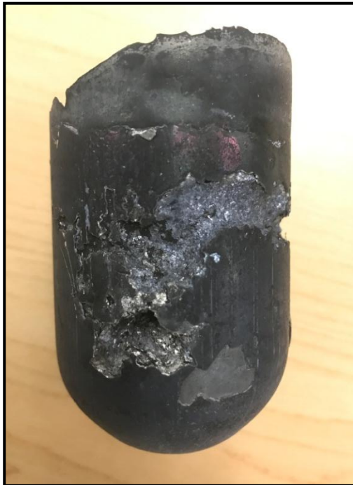
Figure 20: Defective Mg/MWCNT composite due to improper layering of MWCNTs
