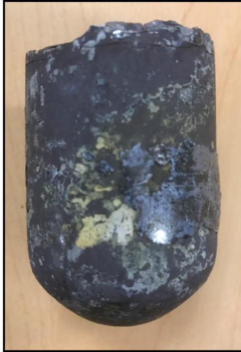
Figure 22: As-cast Mg/MWCNT Billet.
