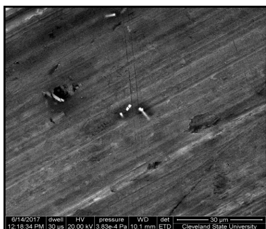
Figure 30: Embedded MWCNTs in Magnesium matrix
