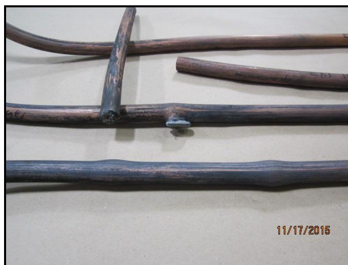
Figure 18: Exploded Cu-Mg/MWCNT composite rod.
