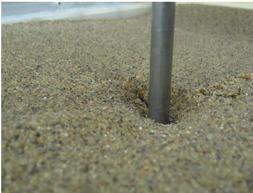
Figure 33: Erosion around cylinder in test section.
