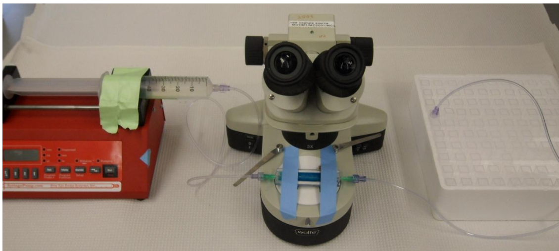
Figure 3.3. Experimental setup. Water is pumped through hydrogel device and collected in cuvettes.
