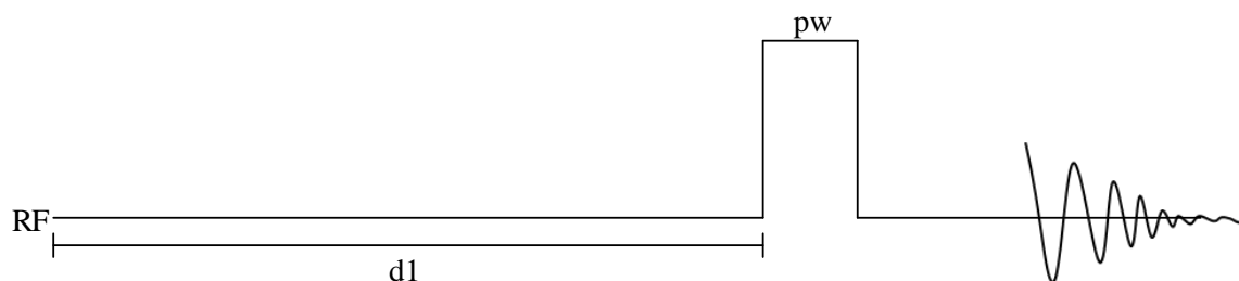
Figure 3.4. One pulse NMR sequence used to generate spectrum
