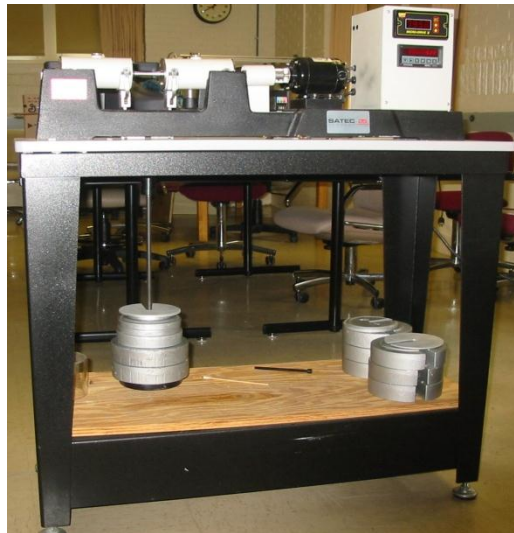
Figure 5-4. The Instron RR Moore rotating fatigue testing apparatus used in this study.
