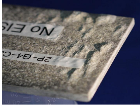
Figure 4-31. An example of exfoliation on the back of a sealed sample
