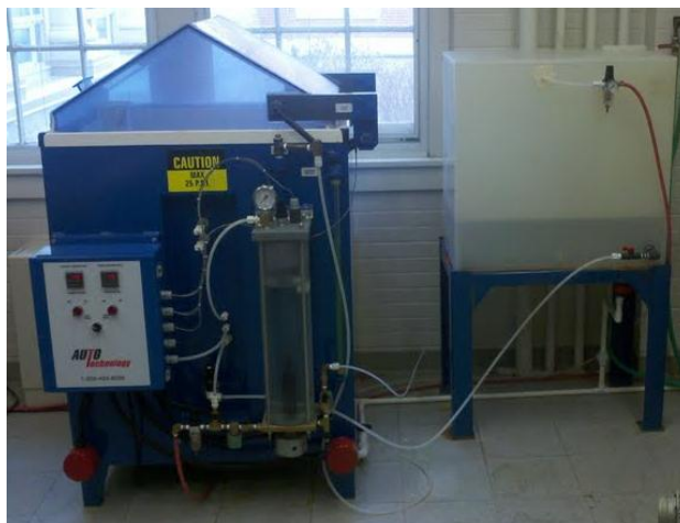
Figure 4-1. The salt spray cabinet (left) and solution chamber (right).
