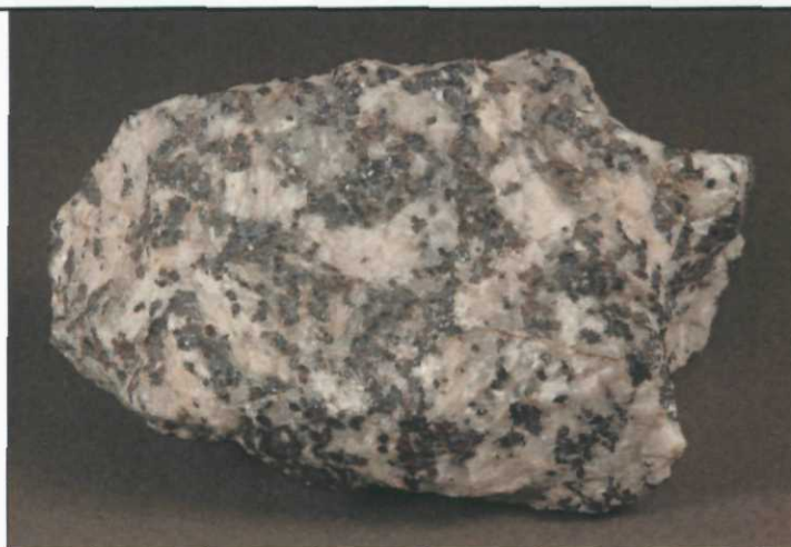
Figure 1. Lean franklinite-calcite-sphalerite ore from the Edison Tunnel – Landmesser Decline area at Sterling Hill, daylight view. Specimen measures 9 x 5 x 5 cm. E.R. Verbeek specimen and photo.
