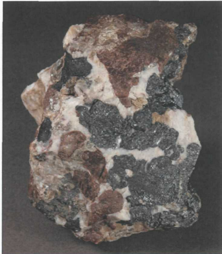
Figure 5. Coarse-grained franklinite-willemite-sphalerite-calcite ore from the North Ore Body, Sterling Hill. Specimen measures 7 x 5.5 x 5 cm. Jim Van Fleet specimen; E.R. Verbeek photo.
