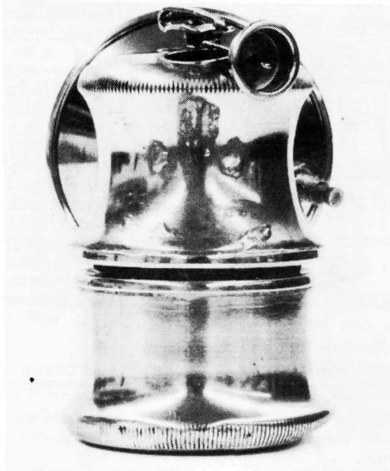
1921 Wolf, back view showing solder traces and water door arrangement
