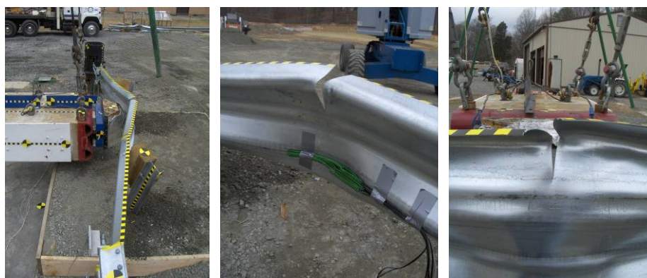
Fig. 12. Test 08-2: Overall damage (left) and detail views of the additional tearing caused by the pendulum impact (center and right)
