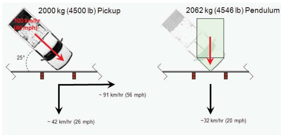
Fig. 5. Comparison of NCHRP 350 (left) and pendulum impact (right) scenarios
