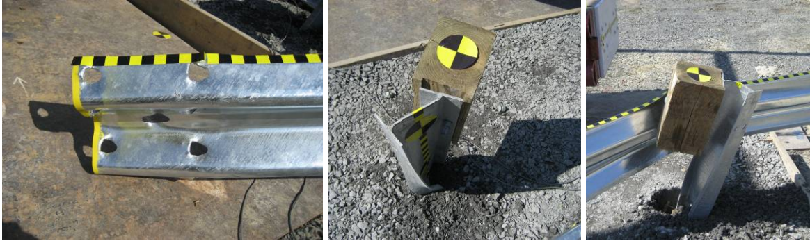
Fig. 15. Test 02-1: Detail view of splice failure (left) and post damage at splice (center) and non-splice location (right)
