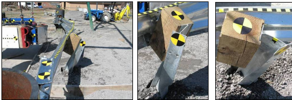
Fig. 6. Test 03-2: Overall damage (right) and post damage at splice (center) and non-splice location (right)
