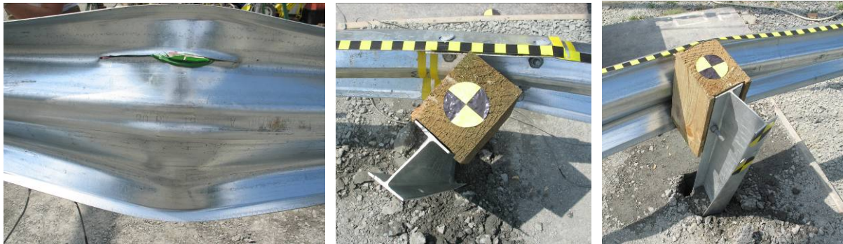
Fig. 13. Test 07-3: Detail view of impact location (left) and post damage at splice (center) and non-splice location (right)
