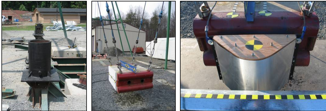
Fig. 2. Existing rigid posts (left), FOIL pendulum mass (center), and new impactor face (right).
