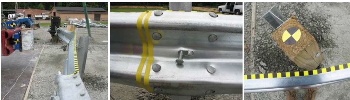
Fig. 20. Test 07-5: overall damage (left), detail view of damage at splice (center) and post damage at non-splice location (right)
