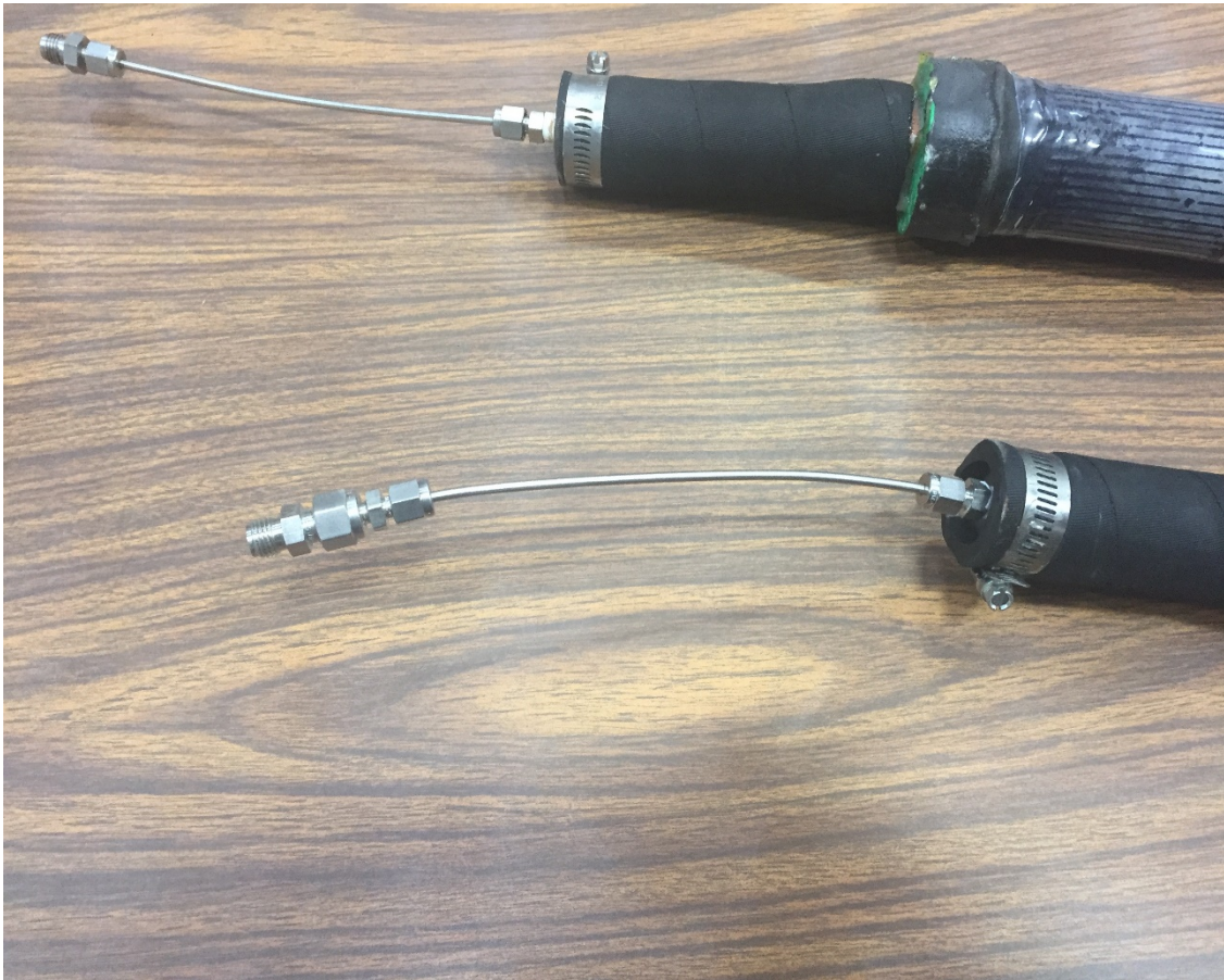
Figure 17 – Photograph of constructed core ends with inflow and outflow tubes attached.
