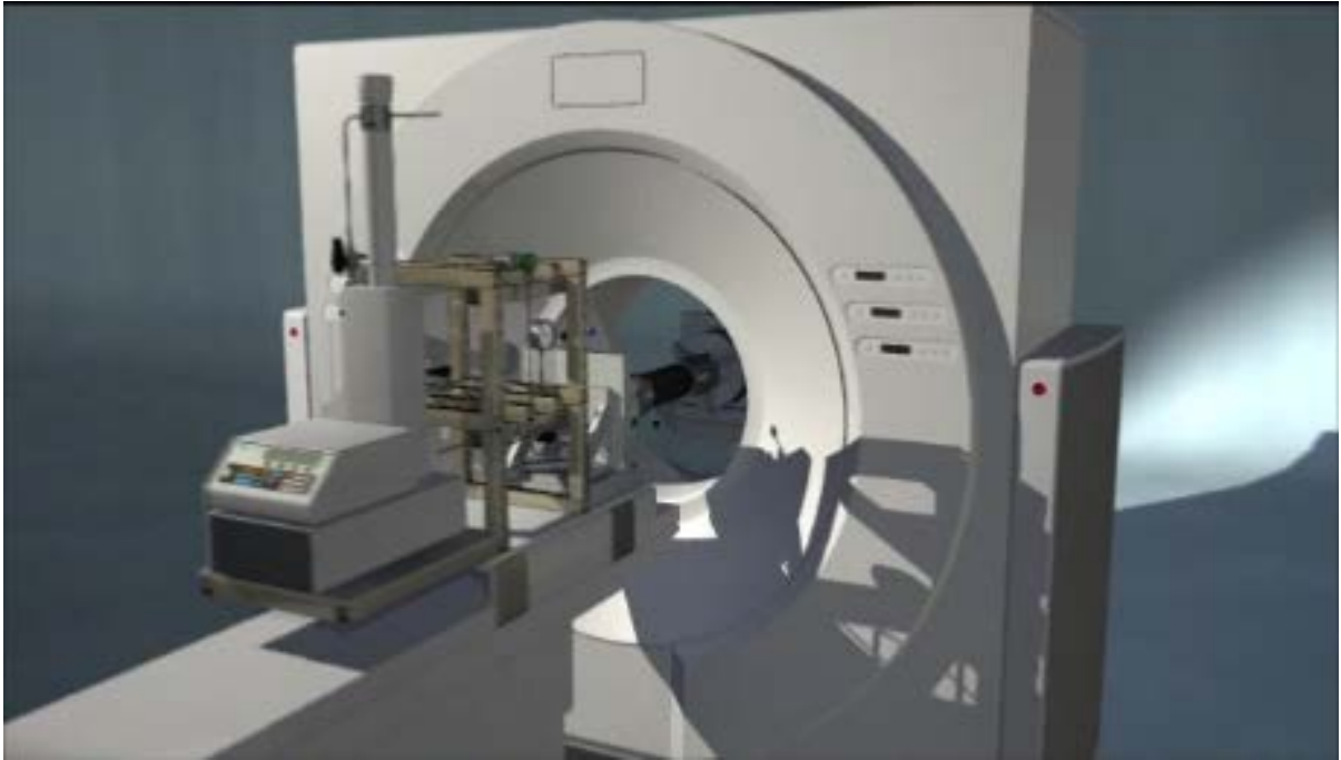
Figure 19 - Cartoon of XRCT scanner. Sample is black cylinder in the middle of the detector donut. The flow control apparatus is outside the donut-shaped detector (NETL).
