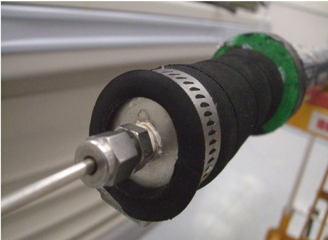
Figure 16 - Photograph of completed core and with attached 1/8" inflow tube. Green areas are core. Everything has been wrapped in Teflon and plastic to seal the conduit (Moore 2016).
