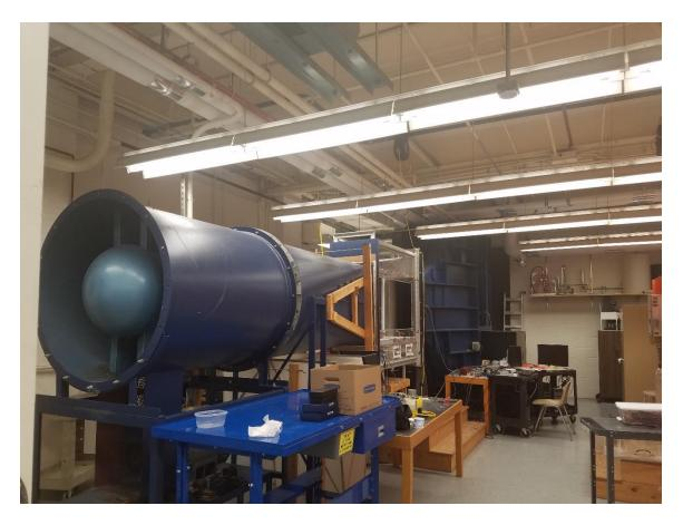
Figure 8 The subsonic open loop wind tunnel in the Mechanical Engineering Laboratory at Bucknell University
