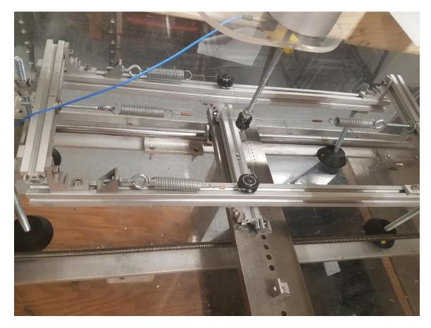
Figure 14 Mounted system with base, threaded rod, cylinder and springs
