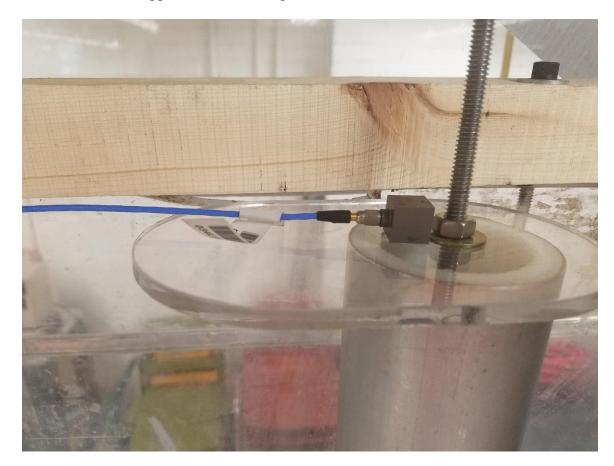
Figure 18 Top accelerometer positioned on the cylinder end plate
