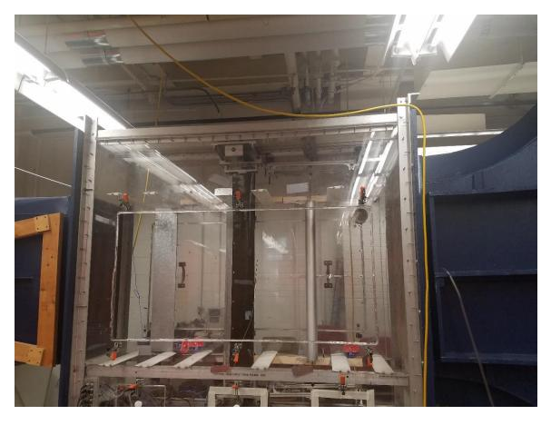
Figure 15 System mounted inside the wind tunnel test section Two steel support bars were designed, manufactured and mounted to the top and bottom of the wind tunnel, connected to each of these bars a structure composed by T-slotted framing aluminum was mounted. The T-slot frame was chosen as it allowed for easy translation of the cylinder in the lift direction without changing its relative position in the stream wise direction.
