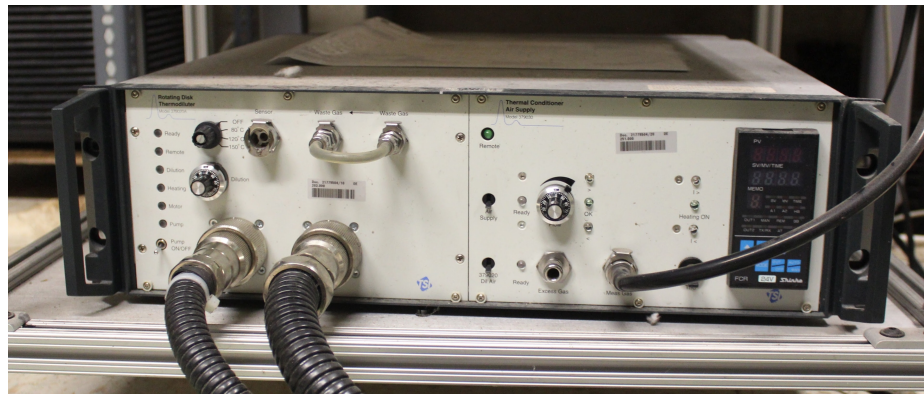
Figure 3.19: TSI 397030 thermal conditioner.
