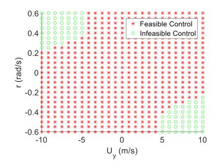
Figure 27. Slice of 3D phase portrait, showing feasible regions of control at U<sub>x</sub> = 10 m/s, for R = 110 m,  $\mu$  = 0.4,  $K_r$  = 28,  $K_\beta$  = 50, and  $K_{U_x}$  = 0.02.
