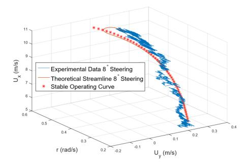
Figure 15. Comparison of experimental and theoretical data for  $8^{\circ}$  steering without braking ( $\kappa = 0$ ) for a stable case.
