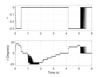
Figure 36. Sequence of steering and braking inputs for a vehicle navigating a 110 m corner with hierarchical sliding surface control.
