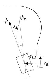
Figure 29. Position of the vehicle relative to the roadway path.
