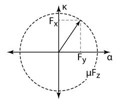
Figure 9. Combined tire force limit.
