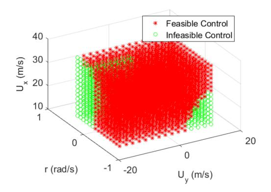
Figure 26. Feasible regions of control in the 3D phase portrait for a 110 m cornering radius,  $\mu = 0.4$ ,  $K_r = 28$ ,  $K_\beta = 50$ , and  $K_{U_x} = 0.02$ .
