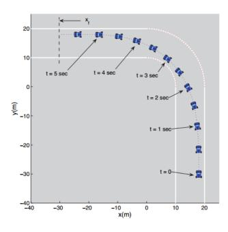
Figure 6. Vehicle trajectory for minimum time cornering maneuver [Velenis 2008].
