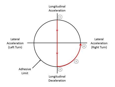
Figure 2. g-g Diagram illustrating the racing line of an expert racecar driver employing the trail braking technique.
