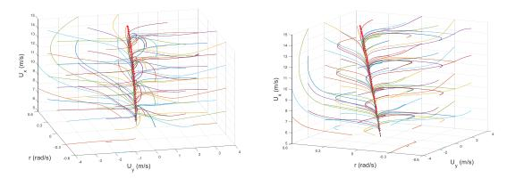
Figure 12. Vehicle stability in the 3D phase portrait for 3° of steering with braking.  $\kappa = -0.05$  and  $\mu = 0.7$ .
