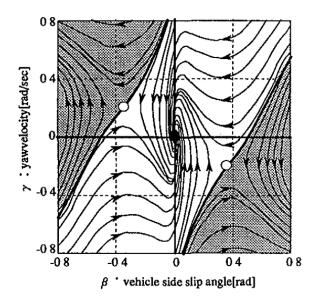
Figure 4.  $\beta - \gamma$  state-plane trajectory at  $U_x = 150$  km/h,  $\delta = 0$  rad [Inagaki 1994].
