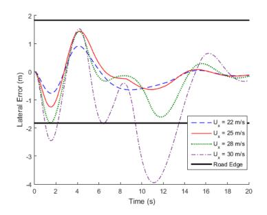
Figure 34. Vehicle lateral error from roadway centerline for various initial longitudinal velocities.  $\mu = 0.4$ , R = 110 m,  $U_{y,initial} = 0$  m/s, and  $r_{initial} = 0$  rad/s.
