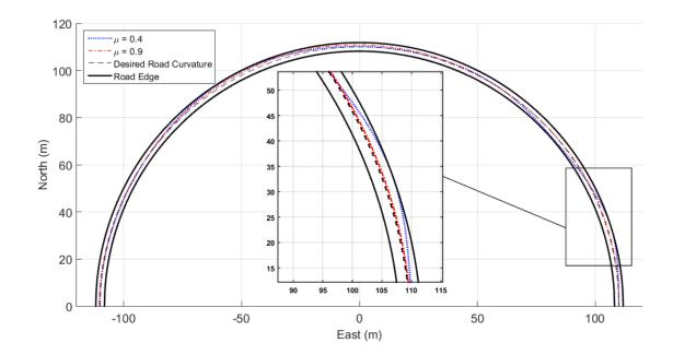
Figure 32. Vehicle response for  $\mu = 0.4$  and  $\mu = 0.9$  with sliding surface controller in place.  $U_{x,initial} = 28$  m/s,  $U_{y,initial} = 0$  m/s,  $r_{initial} = 0$  rad/s, and R = 110 m.
