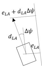
Figure 30. Position of the vehicle relative to the roadway path.  $d_{LA}$  represents the lookahead distance, 10 m.
