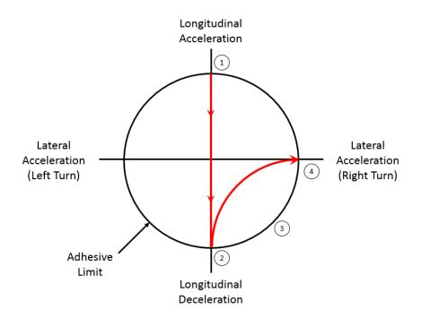
Figure 3. g-g Diagram illustrating an average driver braking and steering through a turn.
