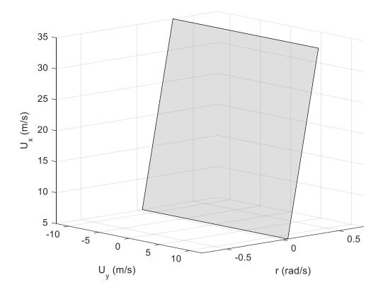
Figure 23. Sliding surface for a cornering radius of 110 m.
