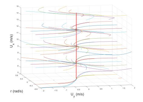
Figure 11. Vehicle stability in the 3D phase portrait for  $0^{\circ}$  of steering and no braking.  $\kappa = 0$  and  $\mu = 0.7$ .
