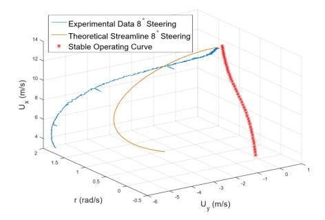
Figure 16. Comparison of experimental and theoretical data for  $8^{\circ}$  steering without braking ( $\kappa = 0$ ) for an unstable case.
