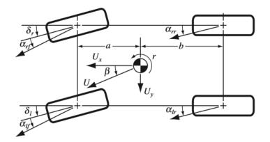
Figure 7. Four wheel planar vehicle model.
