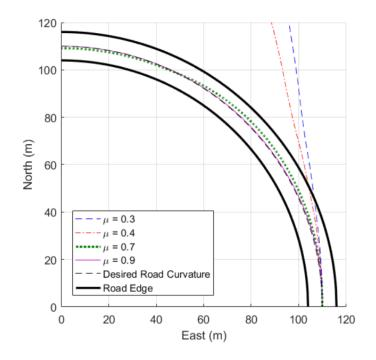
Figure 31. Vehicle response with baseline controller for R = 110 m,  $U_{x,initial} = 28 \text{ m/s}$ ,  $U_{y,initial} = 0 \text{ m/s}$ ,  $r_{initial} = 0 \text{ rad/s}$ ,  $K_e = 0.2$ ,  $d_{LA} = 10$ .
