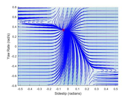
Figure 10. Vehicle stability in the 2D phase portrait for 3° steering,  $U_{x,initial} = 15$  m/s, and  $\mu = 0.75$  with a single stable equilibrium.
