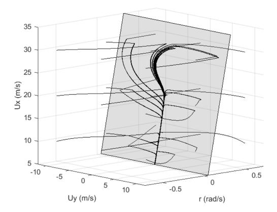
Figure 24. Vehicle trajectories converge to a safe sliding surface.
