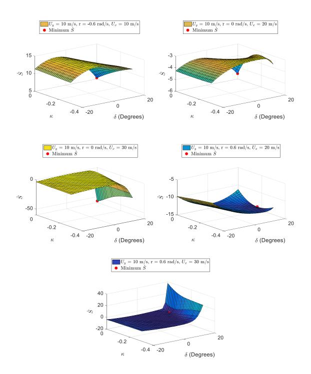
Figure 25. Surface plots of  $\dot{S}$  at several U<sub>y</sub>, r, U<sub>x</sub> vehicle states along with the calculated control inputs indicated in red.
