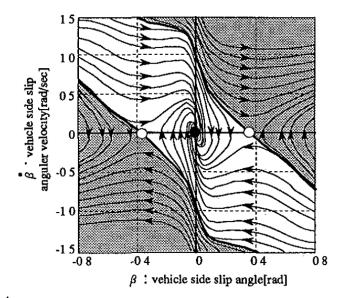
Figure 5.  $\beta - \dot{\beta}$  phase-plane trajectory at  $U_x = 150$  km/h,  $\delta = 0$  rad [Inagaki 1994].
