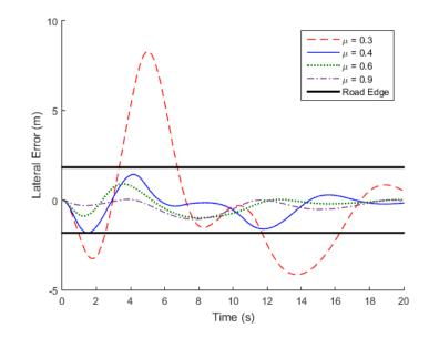
Figure 33. Vehicle lateral error from roadway centerline for various friction coefficients.  $U_{x,initial} = 28 \text{ m/s}, U_{y,initial} = 0 \text{ m/s}, r_{initial} = 0 \text{ rad/s}, \text{ and } R = 110 \text{ m}.$
