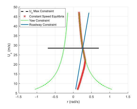
Figure 17. Phase portrait for  $2.5^{\circ}$  steering, no braking, and  $\mu = 0.75$ . Roadway constraint is for a 110 m radius.
