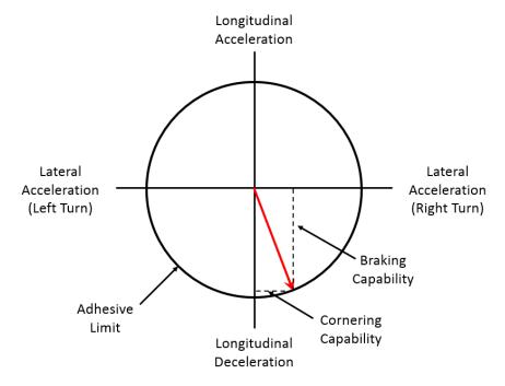
Figure 1. g-g Diagram displaying the acceleration limits of a vehicle.
