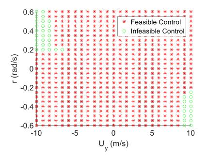
Figure 28. Slice of 3D phase portrait, showing feasible regions of control at  $U_x = 20$  m/s, for R = 110 m,  $\mu = 0.4$ ,  $K_r = 28$ ,  $K_\beta = 50$ , and  $K_{U_x} = 0.02$ .
