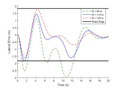
Figure 35. Vehicle lateral error from roadway centerline for various cornering radii.  $\mu = 0.4$ ,  $U_{x,initial} = 28$  m/s,  $U_{y,initial} = 0$  m/s, and  $r_{initial} = 0$  rad/s.
