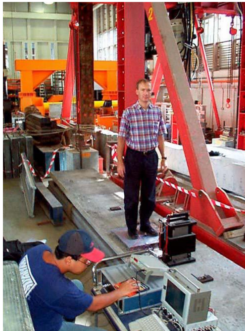
Figure 3: Occupant standing on a precast concrete plank (Brownjohn 1999).
