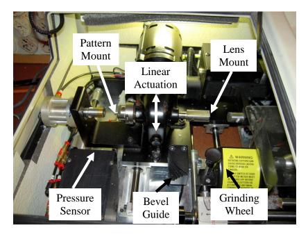
Figure 5-3 Components of Pattern Lens Edger
