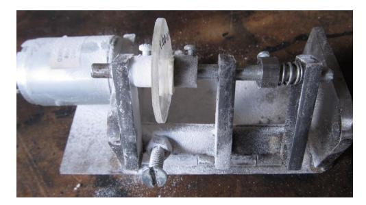
**Figure 5-10 Final Lens Edger Prototype**
