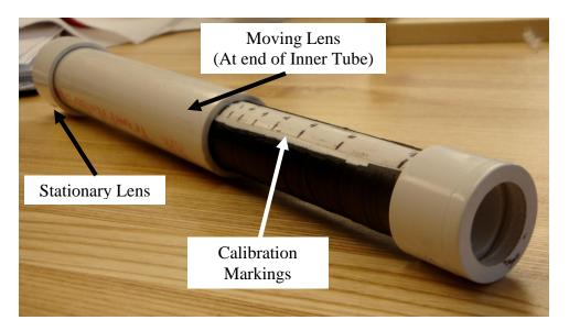
**Figure 5-11 Diagnostic Tool Prototype**
