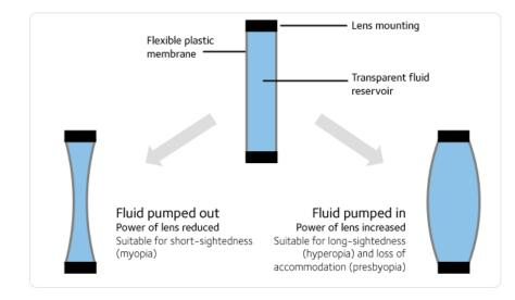
Figure 4-6 Fluid Filled Adjustable Lens Concept [8]
