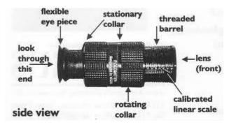
Figure 5-8 Focometer [9]
