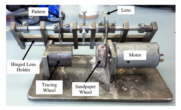
**Figure 5-9 Initial Pattern Lens Edger Prototype**
