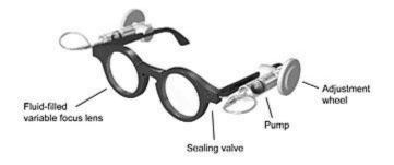
Figure 4-5 Ad-Specs Design [7]
