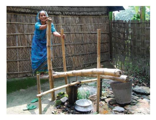
Figure 4-2 IDE Treadle Pump [3]
