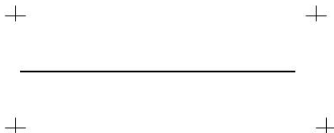
Figure 5.2: Photomask used to imprint a straight channel geometry in a PEG hydrogel microfluidic device system (note: not to scale)
