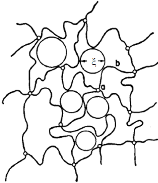
Figure 2.3: Crosslinks (a) between chains (b), and the mesh size, \xi , shown in a crosslinked network 19
