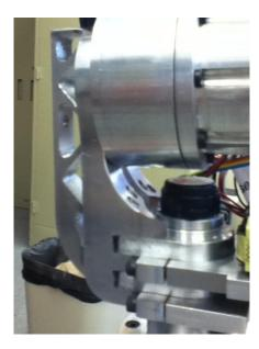
Figure 67: Wrist Bracket Attached Between the Wrist and Elbow
