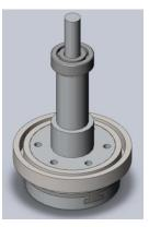
Figure 48: Oldham Coupler with Bearing Placement Shown
