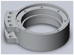
Figure 40: CSD 17 Harmonic Drive Model Figure 41: Lower Case of Elbow Joint
