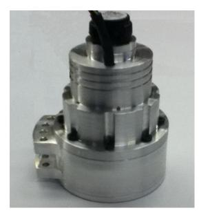
Figure 51: Final Assembled Elbow Joint
