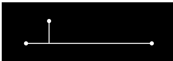
Figure 3.4. T-junction emulsion formation photomask design.
