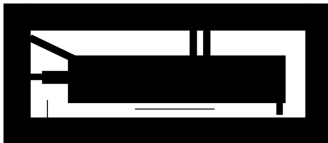
Figure 3.8. Emulsion separation scale-up photomask resulting in ~ 6 mm channel height.
