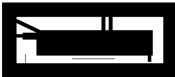
Figure 3.7. Emulsion separation scale-up photomask resulting in ~ 3 mm channel height.
