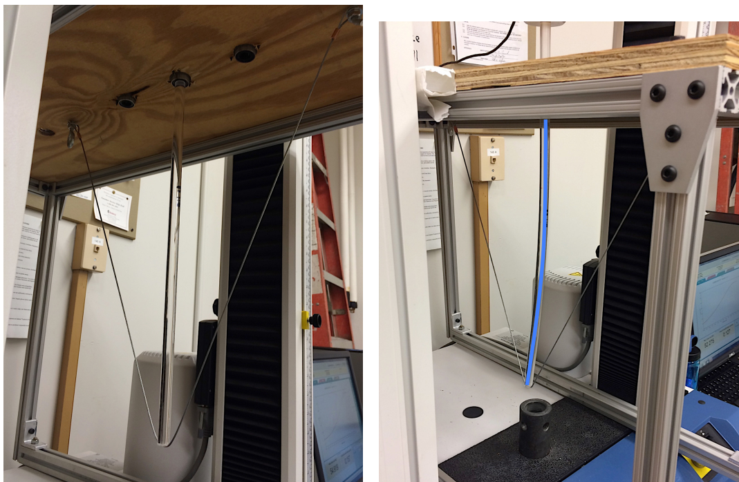
Figure 2.15. Cable apparatus before (left) and after (right) buckling
