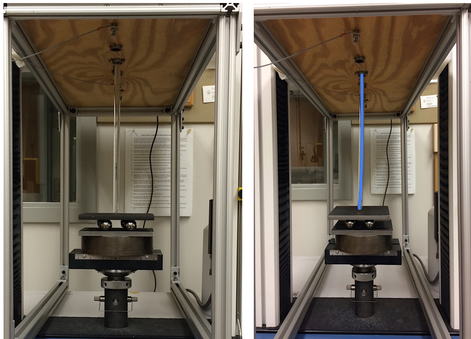
Figure 2.13. Roller apparatus before (left) and after (right) buckling
