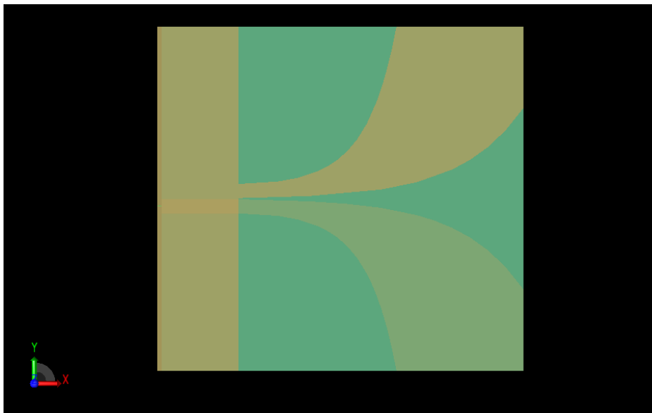
Figure 4.8. Vivaldi antenna modeled in XFDTD 7; opacity is 50%, so the middle conductor curving down is visible.
