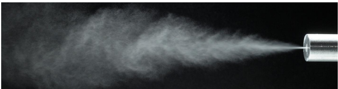
Figure 25. Series of photographs at water flow rate of 12.00 CCM and h = 0.137 in.
