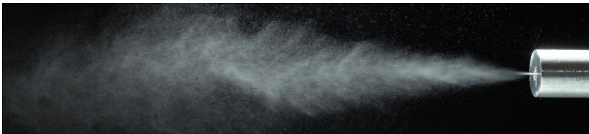
Water: 4.248 CCM, Air: 11.31 LPM, Injector Distance: 0.137 in.
