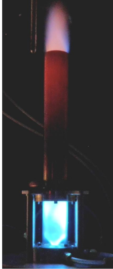
Figure 3. Flame extending past combustion chamber with Delavan injector (adapted from [3]).
