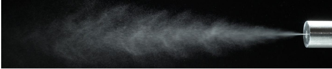
Water: 9.41 CCM, Air: 15.78 LPM, Injector Distance: 0.041 in.
