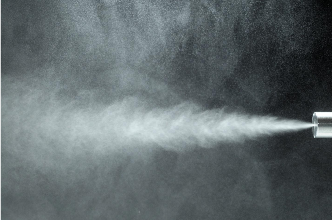
Figure 37. Image of injector at h = 0.029 inches, 14.56 CCM water, and 5.72 LPM air.
