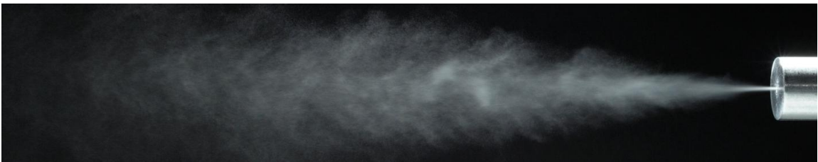
Figure 38. Spray-pattern image at an injector distance of 0.039 inches at 9.41 CCM water and 15.78 LPM air.
