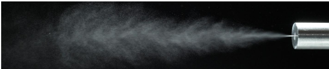
Water: 4.248 CCM, Air: 11.31 LPM, Injector Distance: 0.240 in.
