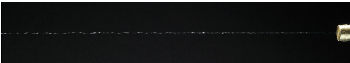
Figure 8. Example of jet breakup using test system.
