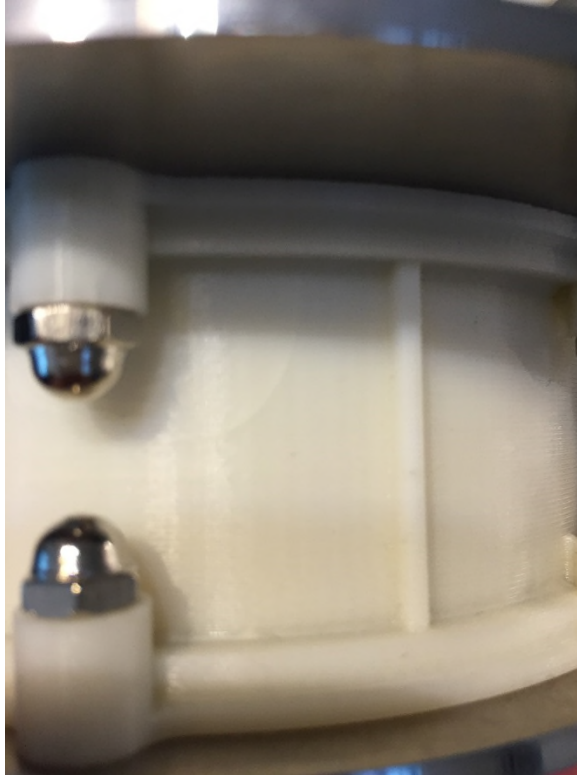
Figure 41. Cracking Around Hot and Cold Plate Mounts
