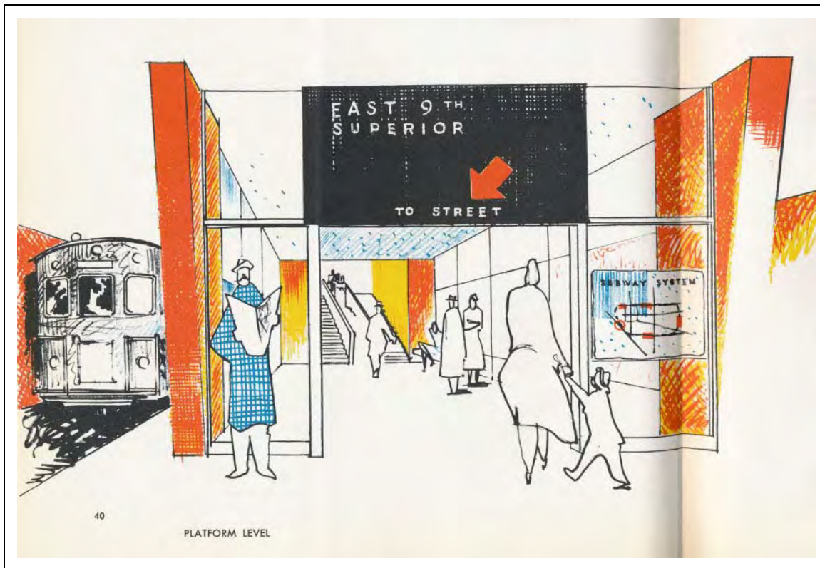
Figure 3. Platform Level, East 9th–Superior Station. Praeger–Cutting–DeLeuw recommended 400-foot-long subway platforms to accommodate eight-car CTS trains. The consultants called for escalators to a mezzanine level, at which they hoped downtown stores would open new subterranean entrances for shoppers. Source: Praeger-Kavanagh, Richard Hawley Cutting & Associates, and Charles E. DeLeuw, Cleveland Subway, Operating and Engineering Feasibility (Cleveland: Board of County Commissioners, Cuyahoga County, Ohio, 1955), 40.
