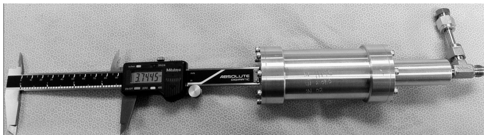
Figure 28: The High Pressure Accumulator and the caliper positioning
