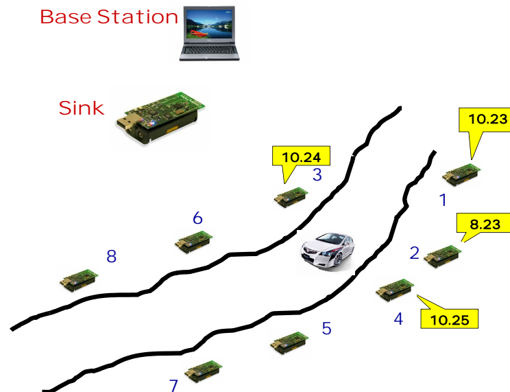
Figure 4: Nodes sense the motion of the car and record their local time at the time of event.
