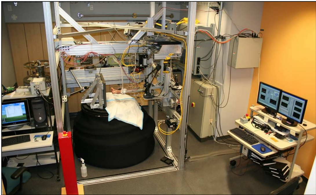
Figure 28 Universal Musculoskeletal Simulator Configured for Foot Studies
