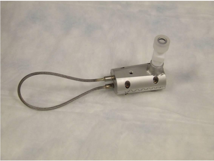
Figure 3 Liquid Nitrogen Distribution System
