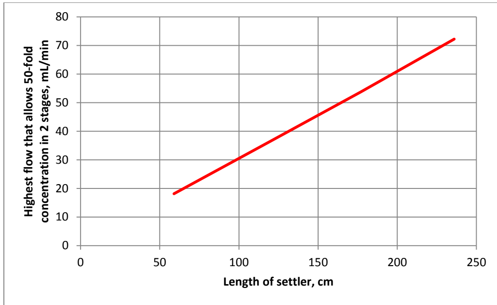
(a) Inlet flow rate vs. settler length at a constant width of 9.6 cm
