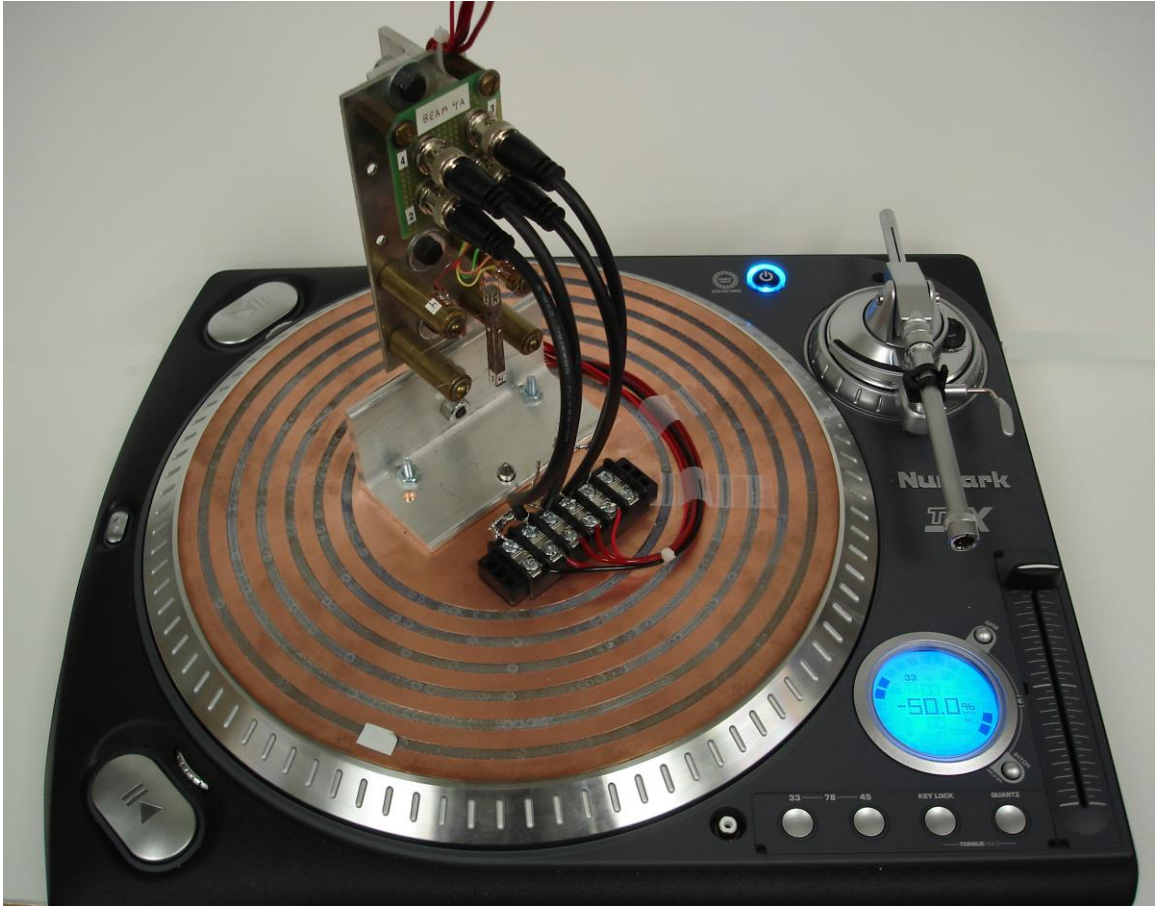
Figure 36: Turn Table with Vibrating Beam Gyroscope
