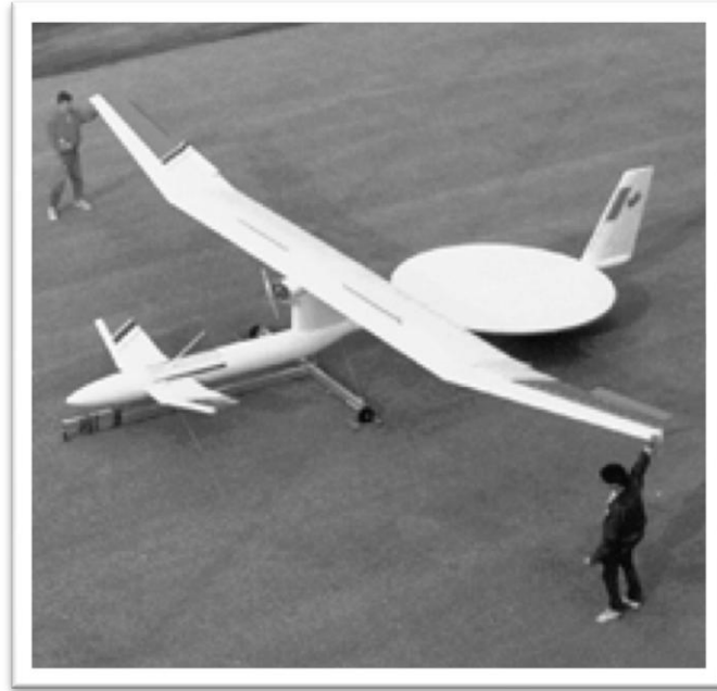
Figure 6: 1/8 SHARP Flight Experiment Model [16]
