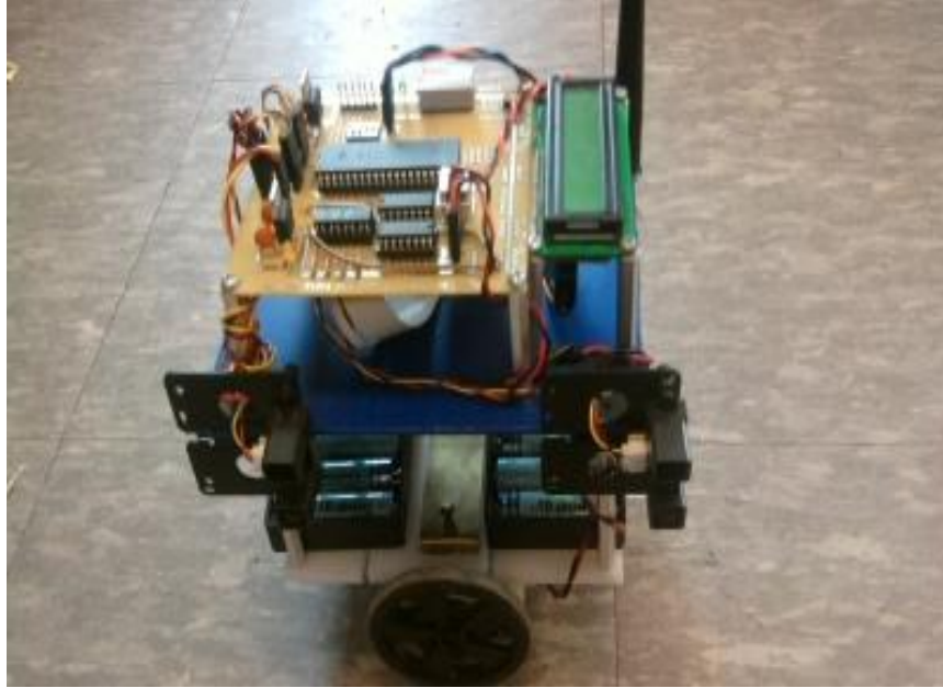
Figure 12: Photograph of the robot. Two IR sensors are seen on the left and right sides of the robot. The wireless radio antenna is seen at the back right side of the photo. The large chip in the middle of the PCB is the PIC18 microcontroller.
