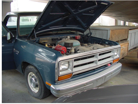
Figure 2. Automotive Stirling engine integrated into a D-150 pickup truck [2]
