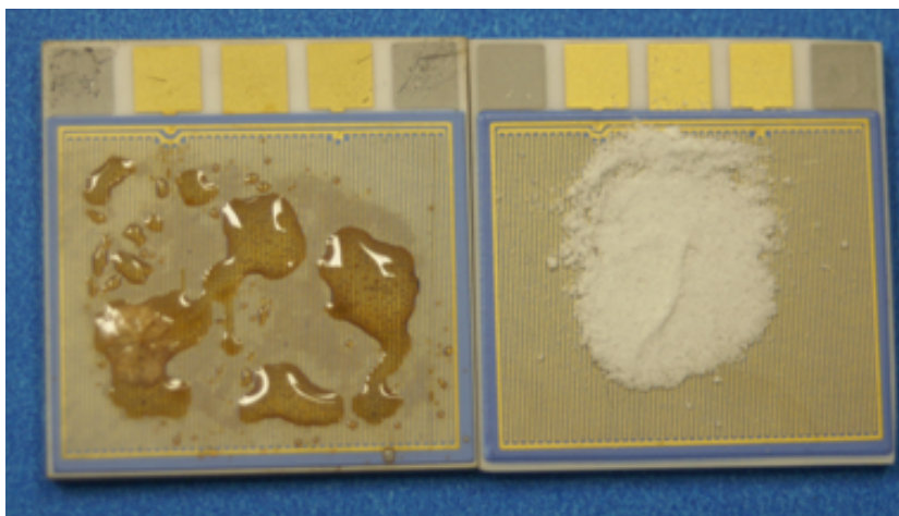
Figure 4.10. Macro photograph of DEA electrodes with sulfa pyridine in Crystalline Powder form (Right), and amorphous form (left) at 2.4 X magnification
