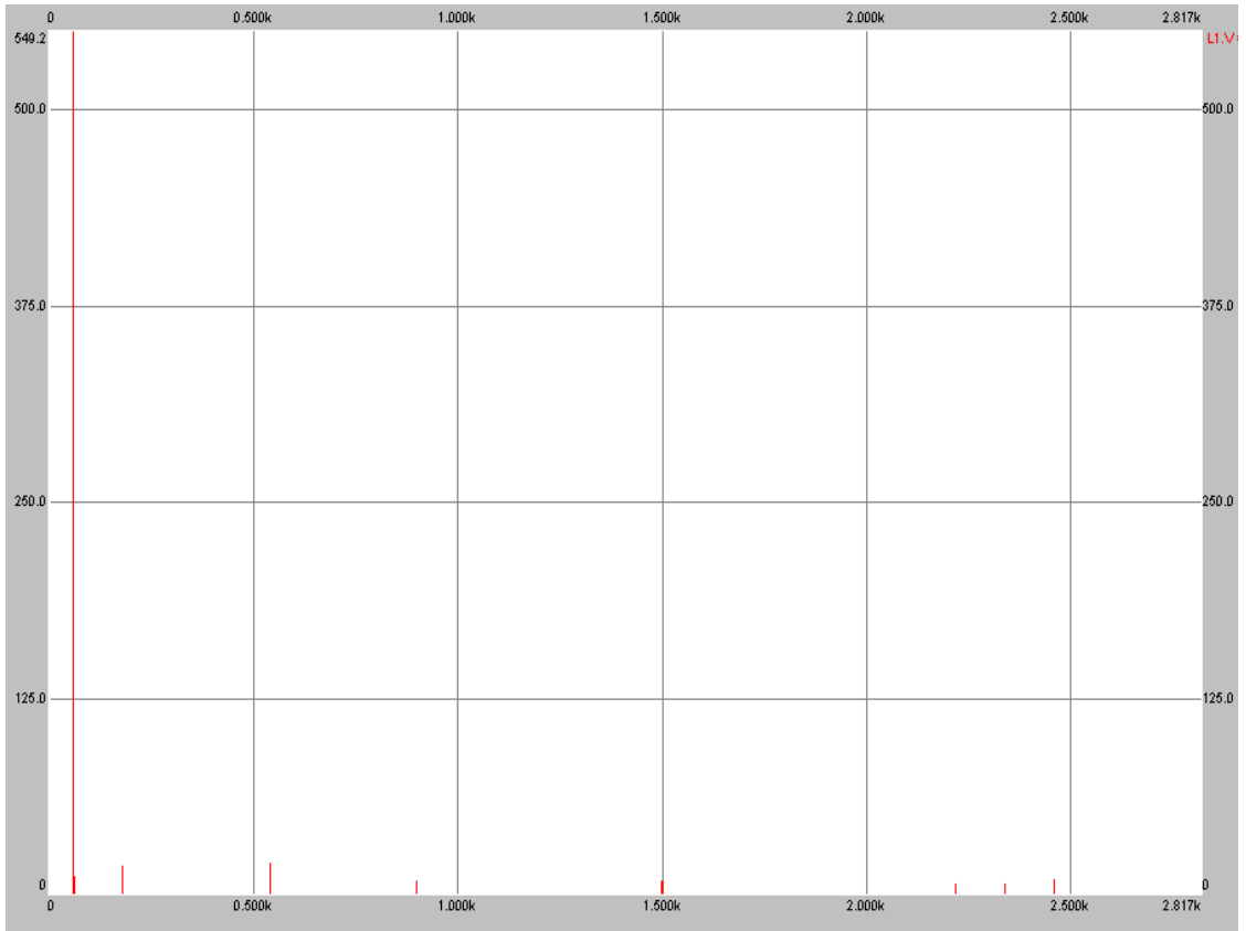
Figure 28: Frequency spectrum for an inductive load
