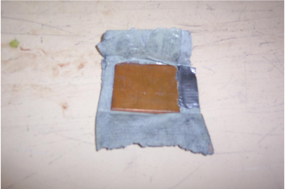
Figure 52: Copper Strips Used for Voltage Detection (Two 1 mm Strips)
