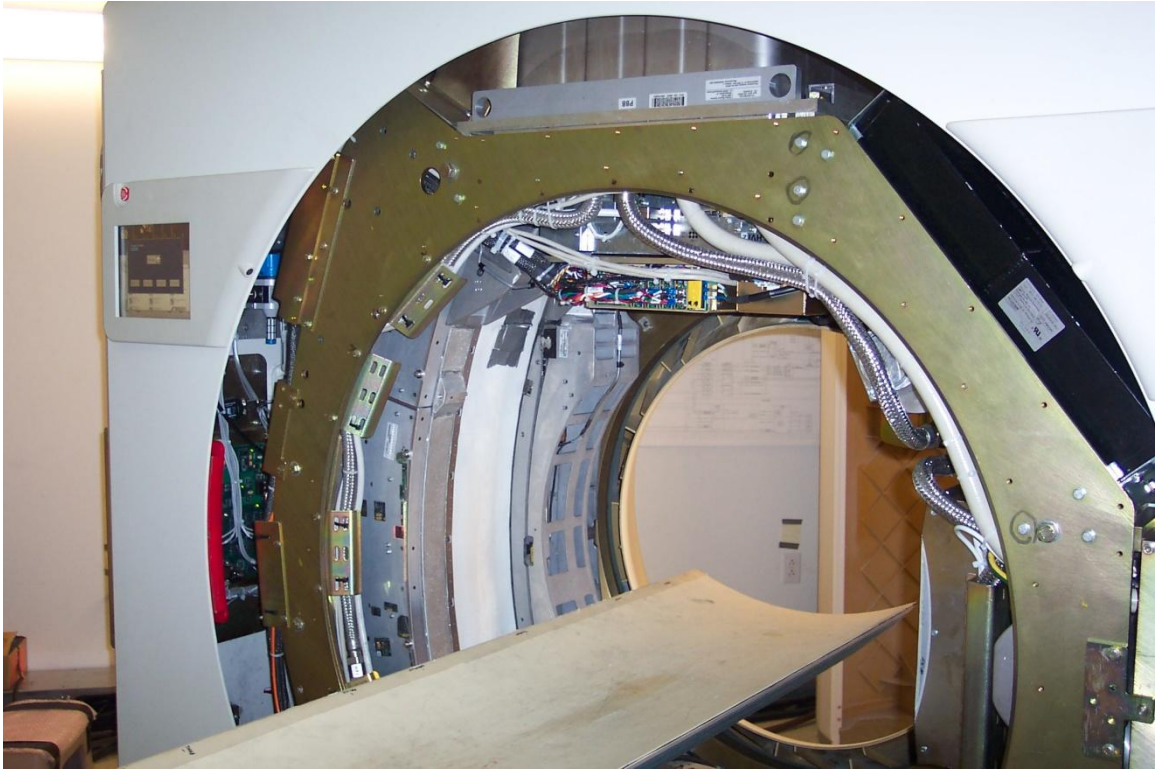
Figure 54: View of System with Copper Strips on Detector Module
